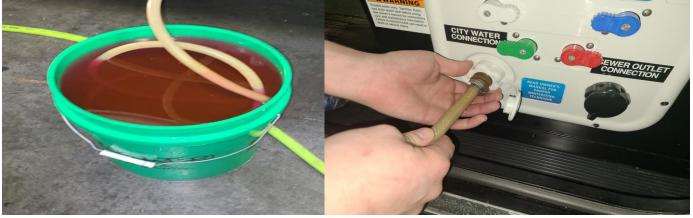
Step 9: go inside the coach and turn on the water pump the pump will begin to pump rv antifreeze into the system the pump will shut off when the system is pressurized
