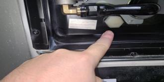
Step:5 remove the water filter cap. Take out the element, dump out water and reinstall the cap tightly
